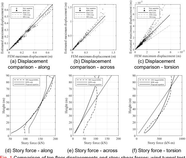
Fig. 1 Comparison of top floor displacements and story shear forces: wind tunnel test, KDS code, and proposed equation
